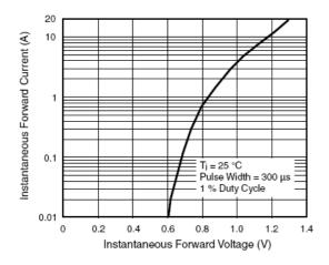
Figure 3. Typical Forward Characteristics Per Diode
