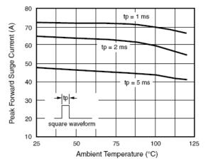
Figure 6. Non-Repetitive Peak Forward Surge Current Square Waveform
