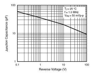
Figure 5. Typical Junction Capacitance Per Diode
